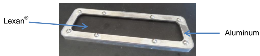
Figure 11 – Tissue Culture Chamber Lid. The lids for the chambers are a two-piece design constructed from Lexan ® polycarbonate and aluminum.
